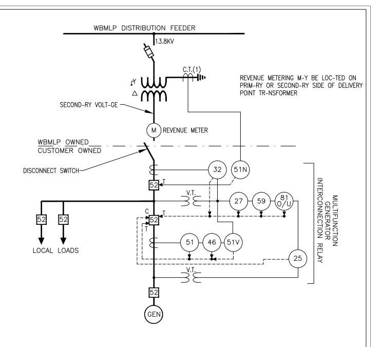
VOLT-GE TR-NSFORMER CONNECTIONS M-Y BE EITHER BROKEN DELT-, SLG DEPENDING ON -PPLIC-TION
